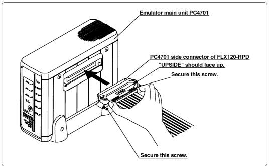
Figure 3.7 Connecting the PC4701 and FLX120-RPD
